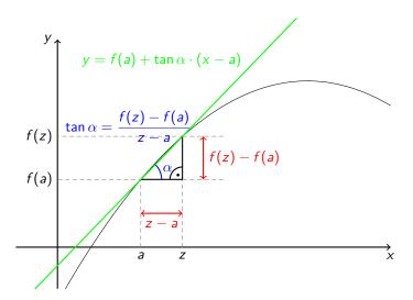
• The tangent line to the graph of a function f(x) at a point  $x_0$  is a straight line that "just touches" the curve at that point.
