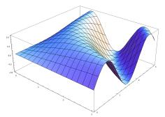
Graph of a two-variable function  $\sin(x \cdot y)$ : the set of points  $(x, y, \sin(x \cdot y))$ .
